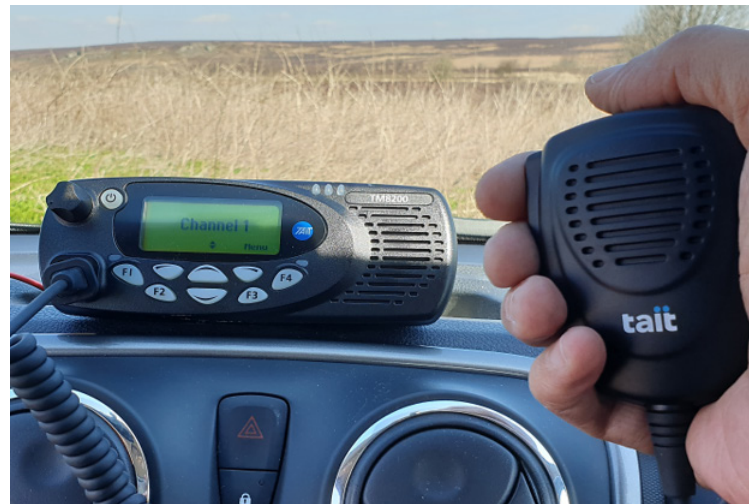
‘dash mounted’ MPT-1327 Mobile Unit (MU) (northern Eurasian location in this example)
