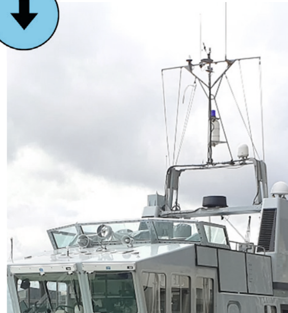
OPV mainmast showing V/UHF communications & intercept antennas
