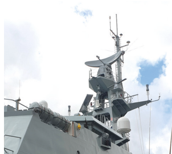
Mainmast with antennas on Offshore Patrol Vessel
