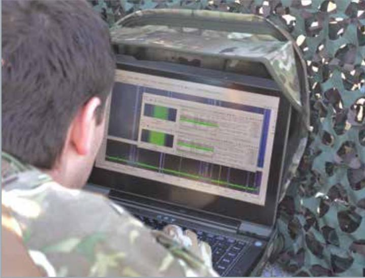
Low Size, Weight and Power ('low-SWaP') communications surveillance systems are becoming ever-more capable. A small laptop PC running go2MONITOR and/or go2DECODE connected to a portable wideband receiver delivers a powerful signals exploitation capability as a light, man-portable or mobile/vehicular system solution, enabling even automatic wideband monitoring with parallel, multi-channel classification and decoding.
